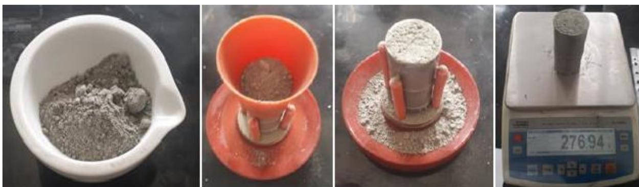
Figure 2. Determination of the bulk density of Amonex.
