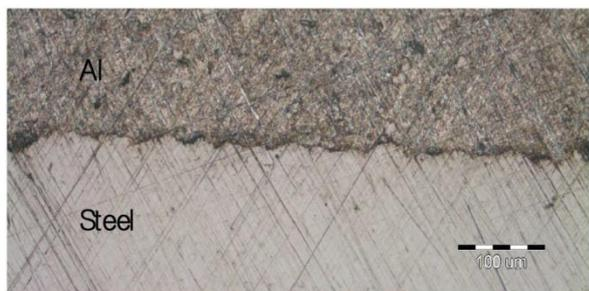
Figure 3. Cross section of the welded material.
