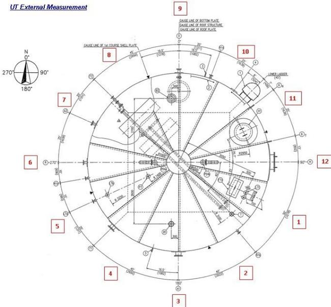
Figure 5. Ultrasonic scheme - cylindrical shell.
