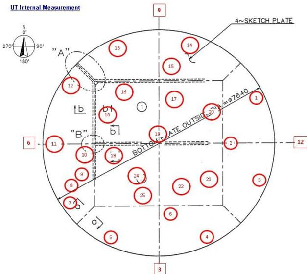
Figure 6. Ultrasonic scheme - tank bottom.
