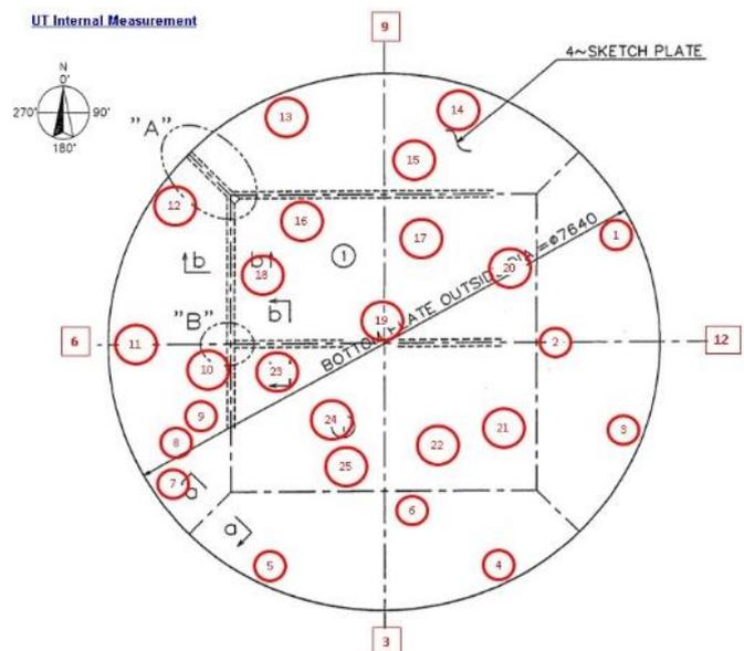
Figure 3. Ultrasonic random scheme for tank bottom overview.
