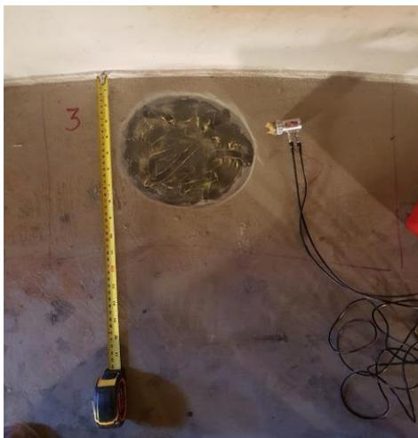
Figure 7. Thickness measuring points according to the created random ultrasonic schemes.
