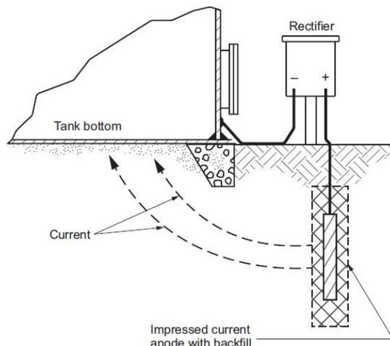
Figure 4. Cathodic protection system with impressed current.
