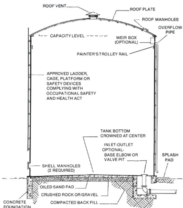
Figure 2. Installation scheme of tank with cone roof.
