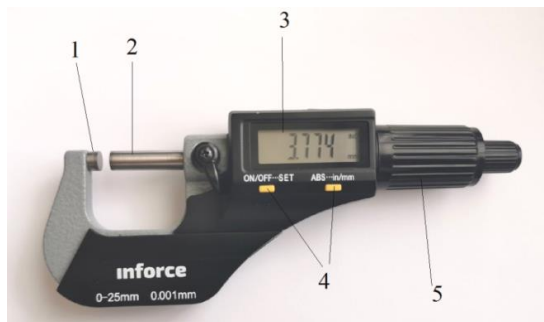
Figure 6. Inforce 06-11-44 digital micrometre: 1-heel of the micrometre; 2-micrometre screw; 3-liquid-crystal display; 4-control buttons; 5-micrometre screw stroke knob.
