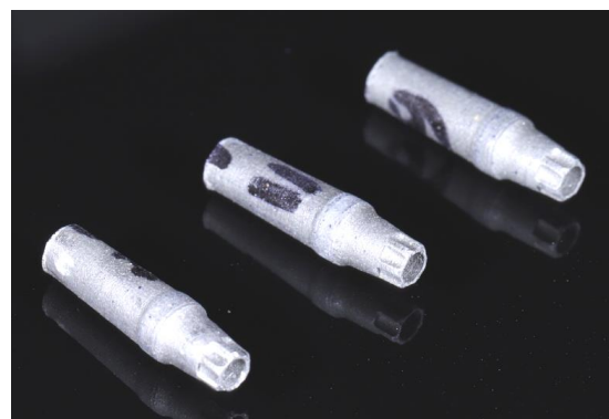
Figure 3. Selective laser sintering abutments with a conical interface for the MISC1 implant.
