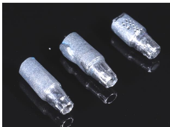
Figure 4. Abutments cast using wax models with a conical interface for the MISC1 implant.
