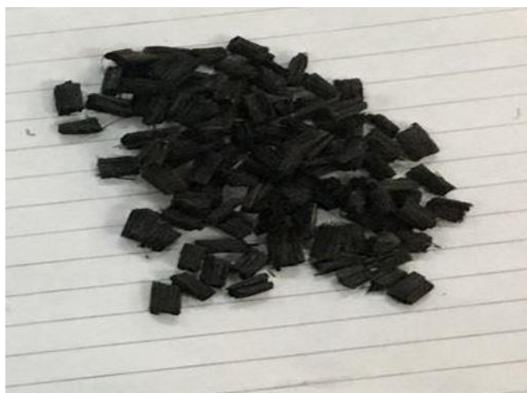
Figure 2. Small pieces of sisal fibre used in the present work.
