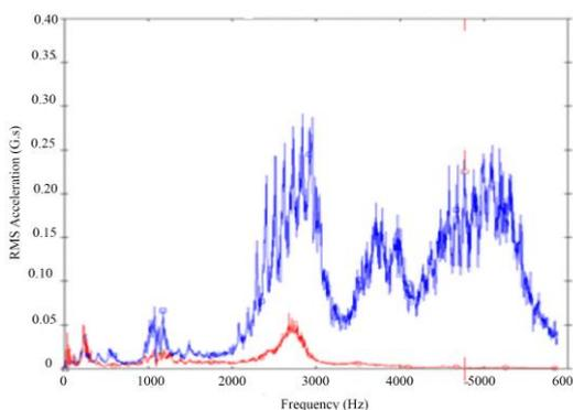
Figure 7. Superposed spectrums with and without lubrication fault.
