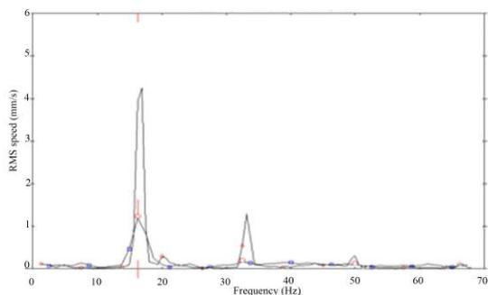
Figure 6. Superposed spectrums with and without fault unbalance.
