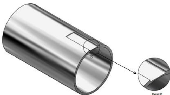
Figure 3. Sectional view of pipeline with corrosion defect (not to scale).
