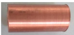
Figure 4. Compression test specimen.
