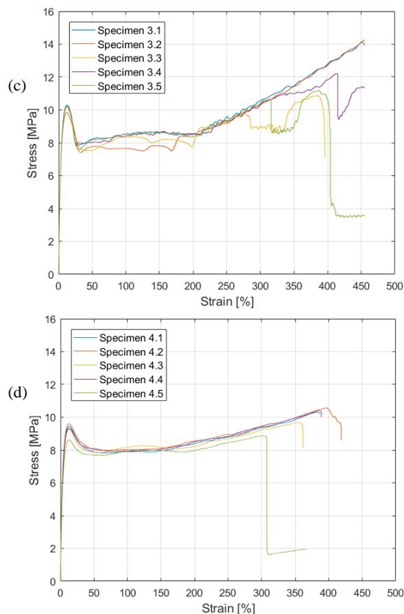
Figure 4. Engineering stress-strain diagrams for: a) 1st batch; b) 2nd batch; c) 3rd batch; d) 4th batch.
