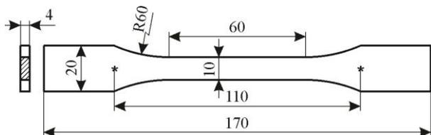
Figure 2. Tensile specimen engineering drawing, according to ISO 527-2:2012, Type 1A (units in mm).
