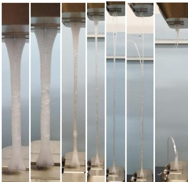
Figure 3. Tensile testing of PP specimen, from start to failure.
