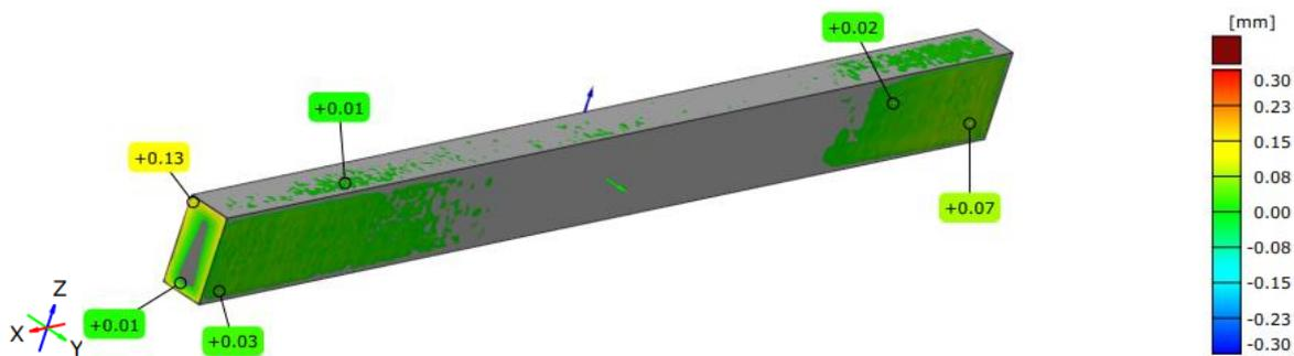
Figure 10. Vertically-oriented bending specimen - upper side.
