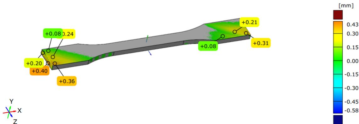
Figure 4. Horizontally-oriented tensile specimen - upper side.
