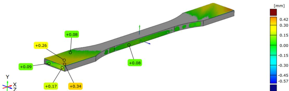
Figure 6. Vertically-oriented tensile specimen - upper side.
