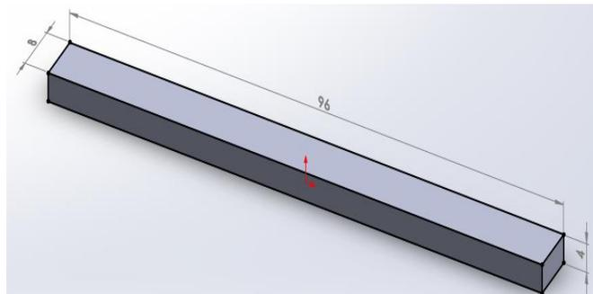
Figure 2. The CAD model of a bending specimen according to /11/
