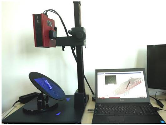
Figure 3. Tensile specimen (up); bending specimen (bottom) - mounted on the device during 3D scanning.
