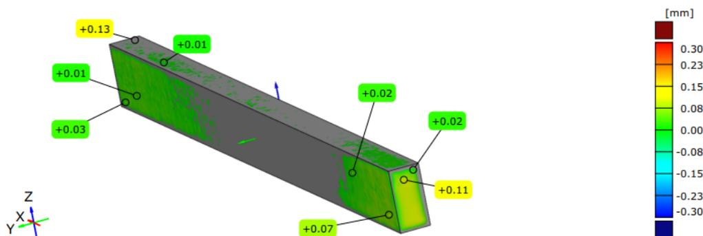
Figure 11. Vertically-oriented bending specimen - bottom side.
