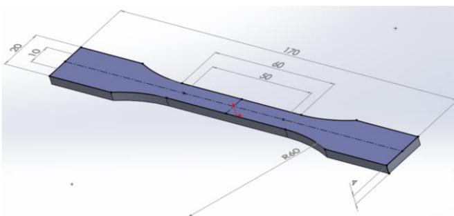
Figure 1. CAD model of tensile Type 1A specimen according to /10/.
