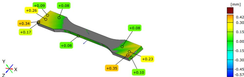
Figure 7. Vertically-oriented tensile specimen - bottom side.
