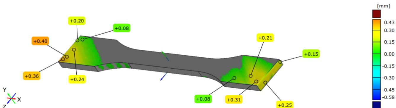
Figure 5. Horizontally-oriented tensile specimen - bottom side.
