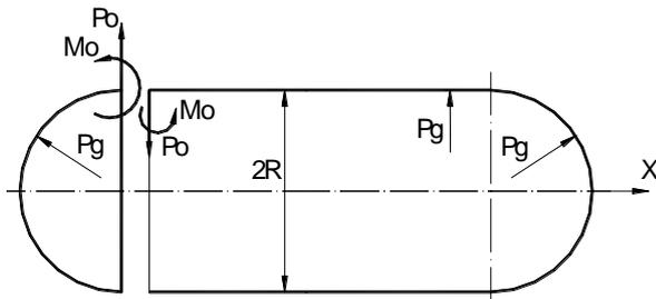
Figure 1. Cylindrical reservoir loaded by internal pressure.
