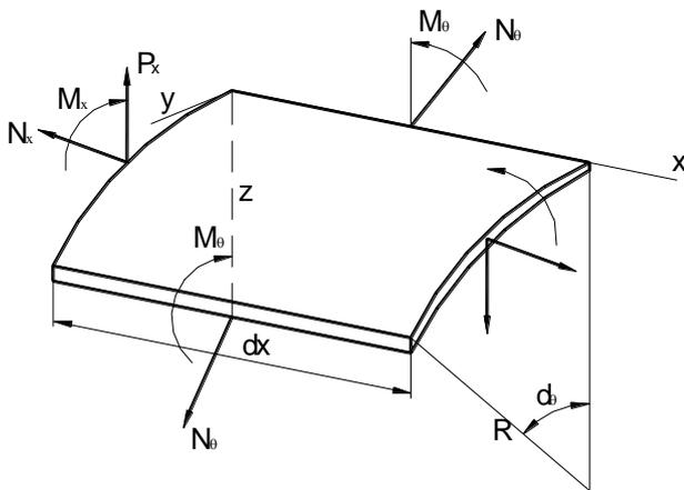
Figure 2. Forces in the cylindrical shell from gas pressure.
