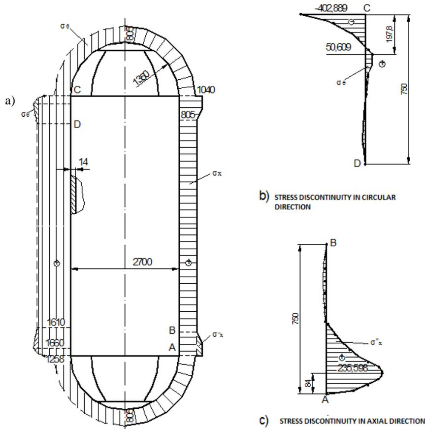
Figure 4. Cylindrical reservoir with ends shaped as hemisphere, loaded only by gas pressure.
