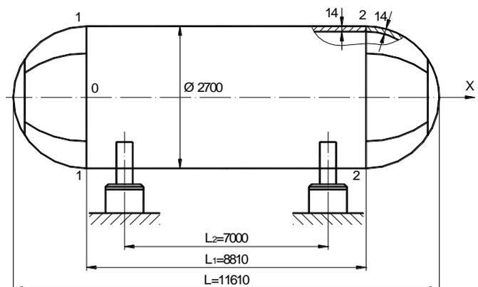
Figure 3. Stable 60 m<sup>3</sup> reservoir for propane-butane gas.
