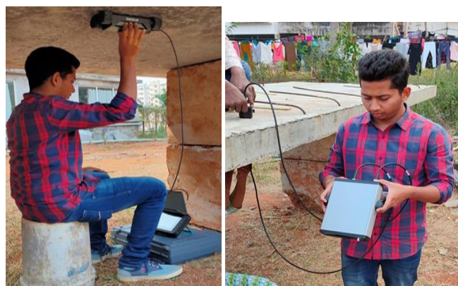
Figure 2. Scanning using Profometer PM-600; concrete quality testing using UPV.
