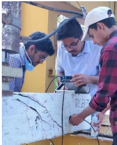
Figure 18. Beam testing under stress condition using NDT.
