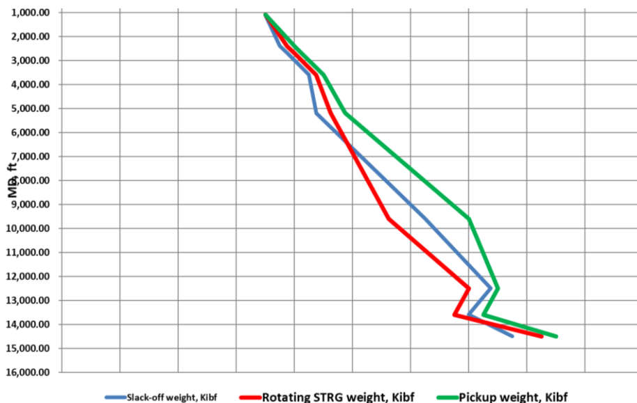
Figure 9. Rotation STRG weight, pick-up weight, slack-off weight vs. measured depth for direction well No.3.
