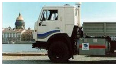
Figure 2. KAMAZ truck, equipped with cryogenic LNG tank of fuel capacity 300 lit.
