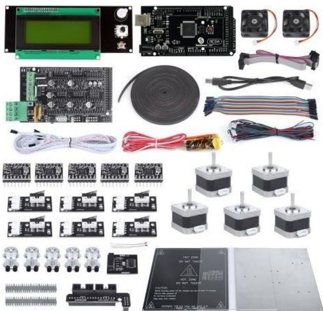
Figure 3. Kit with electronic components for the Rostock 3D printer, /8/.
