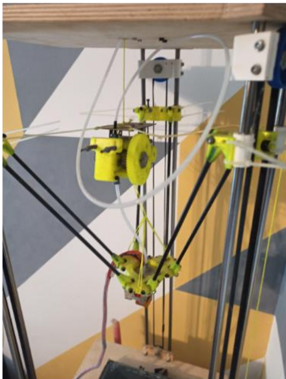
Figure 5. Floating extruder with hot-end (photo and 3D printer made by M. Aleksandrović), /16, 17/.
