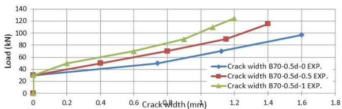
Figure 15. Load experimental crack width of B70-0.5d.
