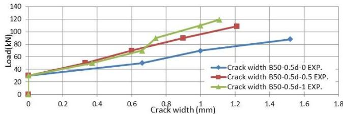
Figure 14. Load-experimental crack width of B50-0.5d.
