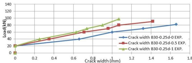
Figure 13. Load-experimental crack width of B30-0.25d.
