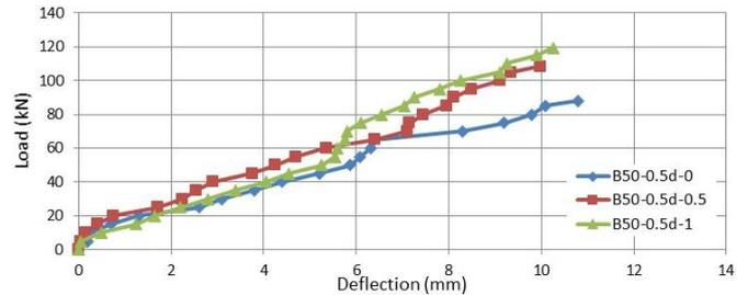
Figure 8. Load vs. experimental deflection, B50-0.5d.
