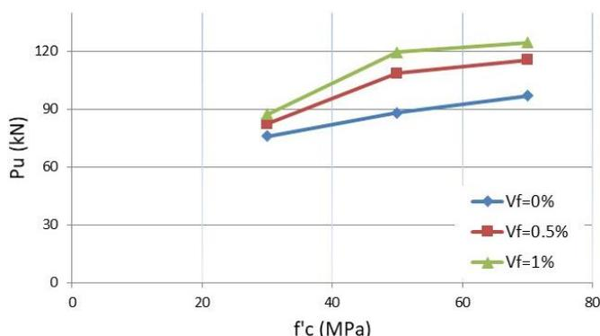
Figure 4. Effect of concrete compressive strength.
