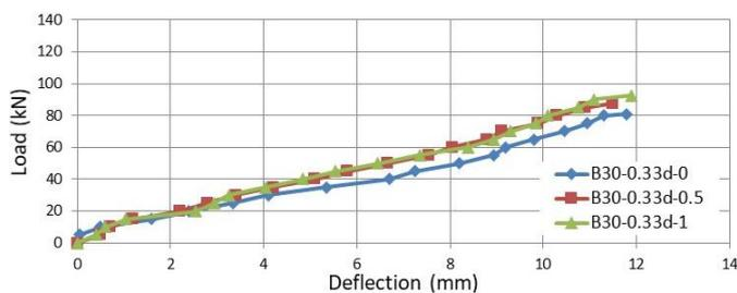
Figure 6. Load vs. experimental deflection B30-0.33d.
