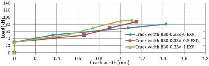
Figure 12. Load-experimental crack width of B30-0.33d.
