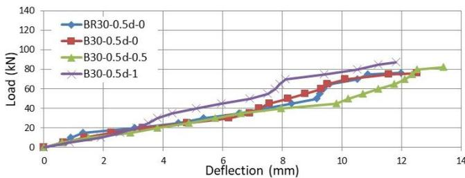
Figure 5. Load vs. experimental deflection B30-0.5d.
