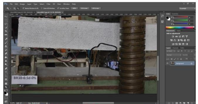
Figure 10. Crack width measurement.
