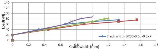
Figure 11. Load-experimental crack width of B30-0.5d.
