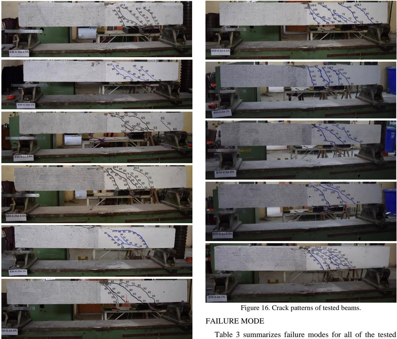
Figure 16. Crack patterns of tested beams.
