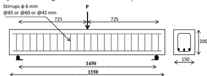
Figure 1. Details of tested beam.
