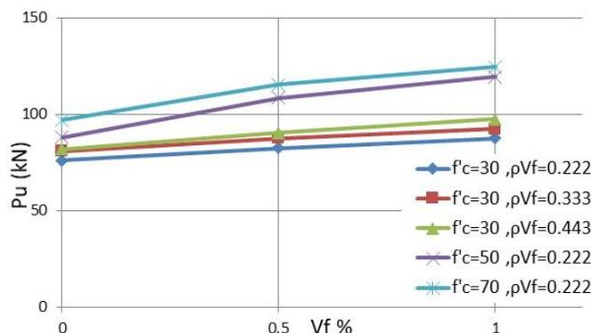
Figure 3. Effects of steel fibres on failure load.
