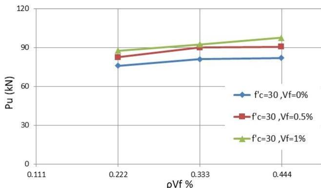
Figure 2. Effect of shear reinforcements on failure load.
