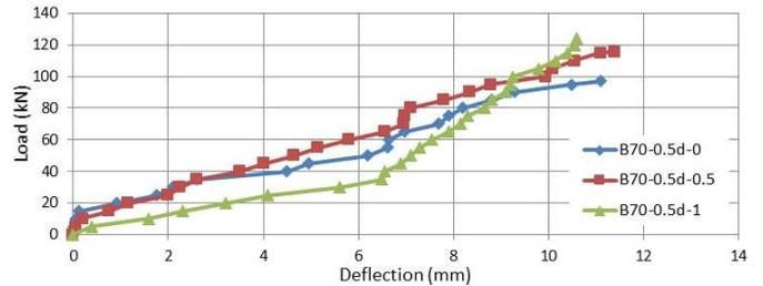
Figure 9. Load vs. experimental deflection, B70-0.5d.
