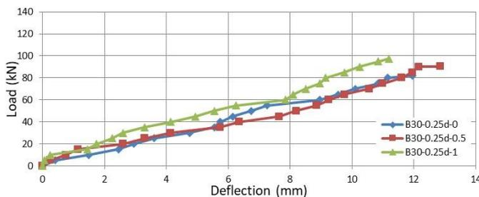
Figure 7. Load vs. experimental deflection B30-0.25d.
