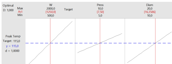
Figure 13. Plots of main effects of parameters on peak temperature.
