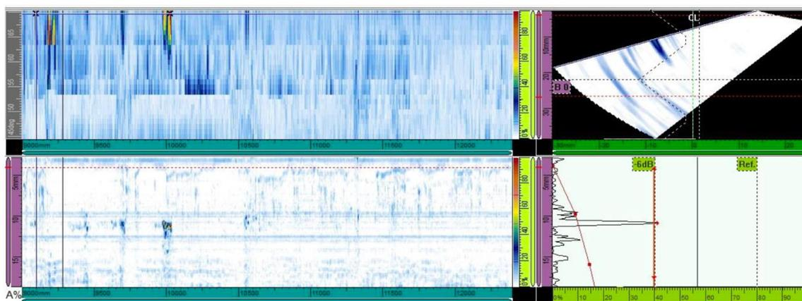
Figure 2. First defect discovered by PAUT at a depth of 9096 mm from the coordinate origin.
