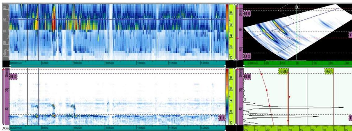
Figure 4. Third defect discovered by PAUT at a depth of 9451 mm from the coordinate origin.
