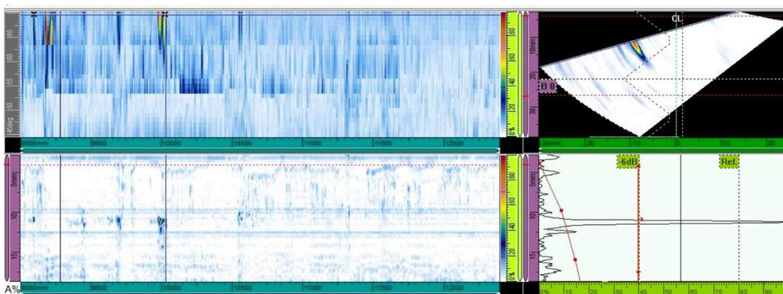
Figure 3. Second defect discovered by PAUT at a depth of 10028 mm from the coordinate origin.
