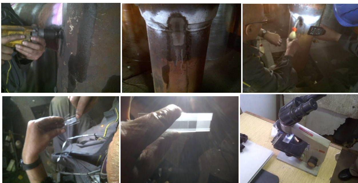
Figure 9. Replica method testing procedure.
