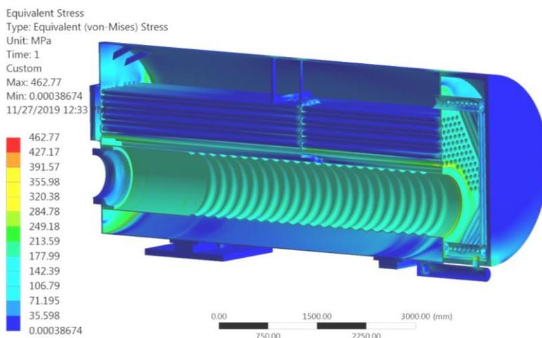
Figure 7. Equivalent stresses of hot water boiler structural elements at 100 s from the moment of starting up the boiler.
