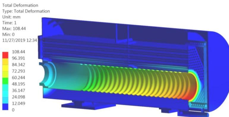
Figure 8. Total deformation of hot water boiler structure at 100 s from the moment of starting up the boiler.
