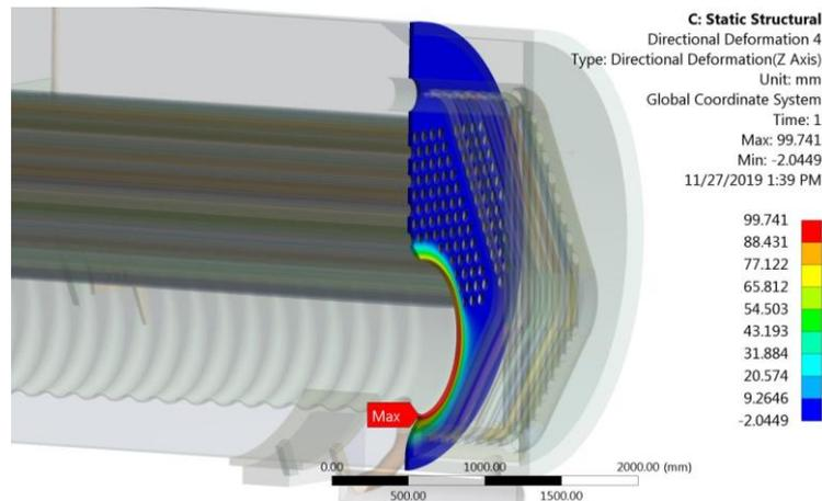
Figure 10. Total deformation (directional Z Axis) of the tube plate of the first reversing chamber at 100 s from the moment of boiler start-up.
