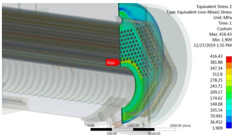
Figure 9. Equivalent stresses of tube plate of the first reversing chamber at 100 s from the moment of starting up the boiler.
