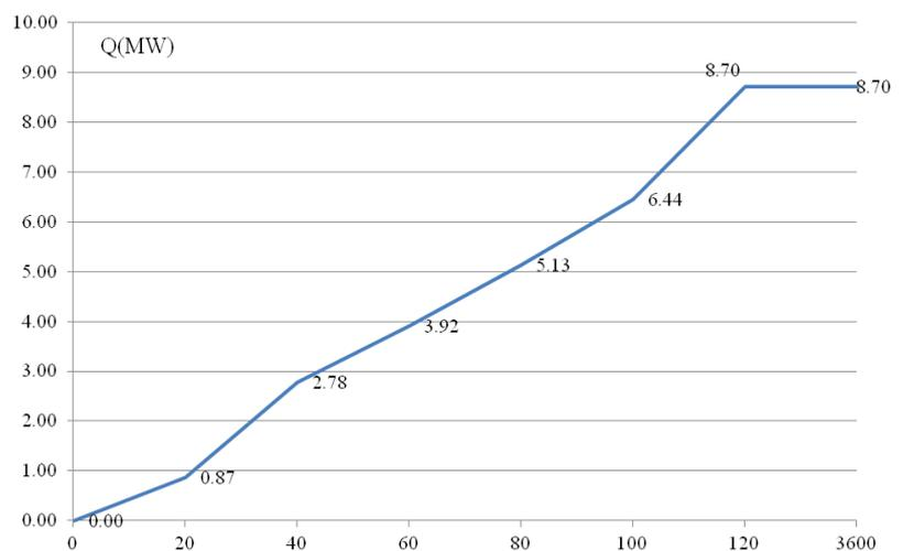
Figure 4. Heat load change of the fire tube  $Q$  as a function of time.
