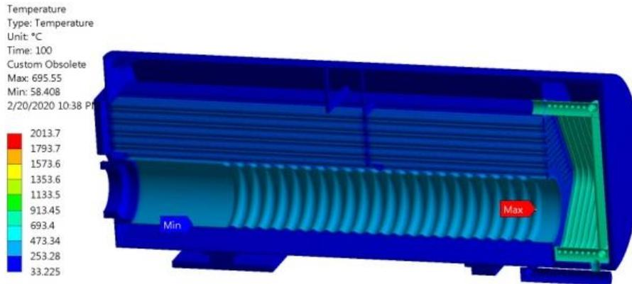
Figure 5. Temperature distribution of boiler elements after 100 s from starting up of the boiler.
