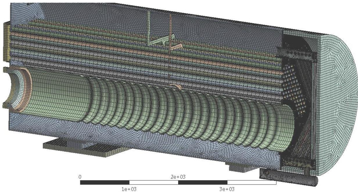
Figure 3. Discretized structure of hot water boiler.
