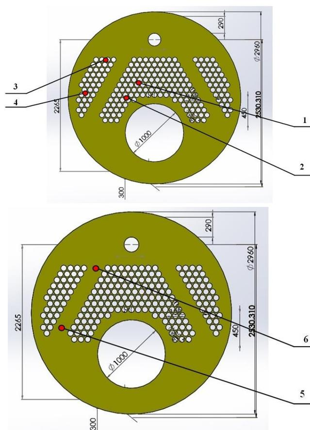
Figure 1. Position of temperature probes.
