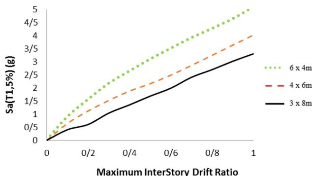
Figure 17. Mean values of IDA curves of four floor frame for spans with various dimension and comp. strength of 23.42 MPa.
