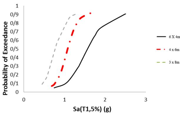
Figure 31. Fragility curves for frames with 4 floor structure with compressive strength of 21 MPa in LS performance level.
