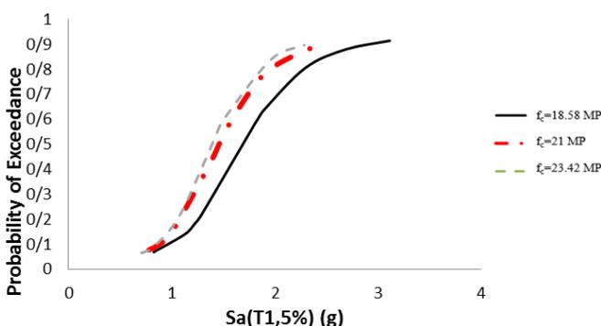
Figure 26. Fragility curves for four floor frame with 3 spans of 8 m in CP performance level.
