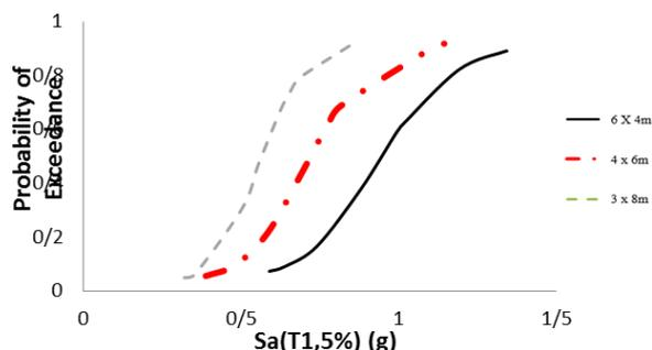
Figure 27. Fragility curves for frames with 4 floor structure with compressive strength of 18.58 MPa in IO performance level.
