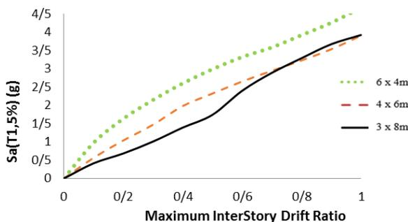
Figure 16. Mean values of IDA curves of four floor frame for spans with various dimension and comp. strength of 21 MPa.
