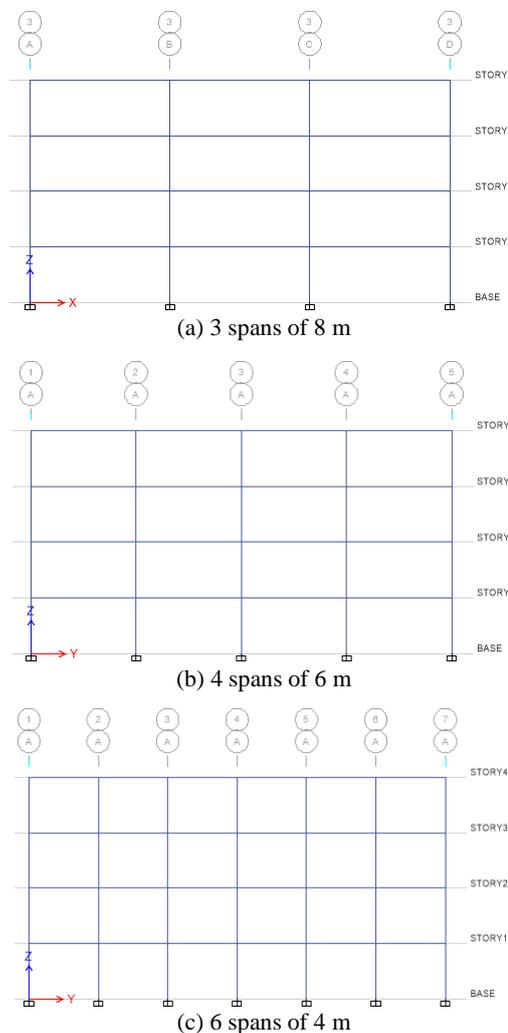
Figure 2. View of 3D structures with various span lengths.
