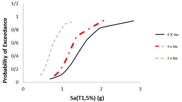
Figure 34. Fragility curves for frames with 4 floor structure with compressive strength of 23.42 MPa in LS performance level.
