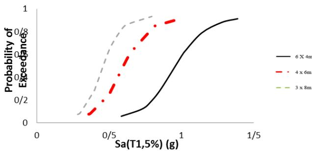
Figure 30. Fragility curves for frames with 4 floor structure with compressive strength of 21 MPa in IO performance level.
