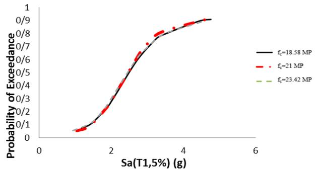
Figure 20. Fragility curves for four floor frame with 6 spans of 4 m in CP performance level.
