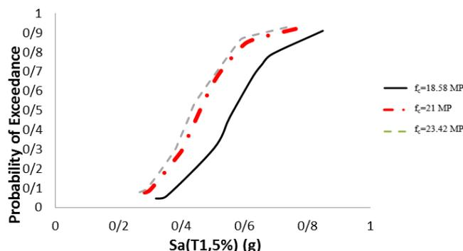
Figure 24. Fragility curves for four floor frame with 3 spans of 8 m in IO performance level.
