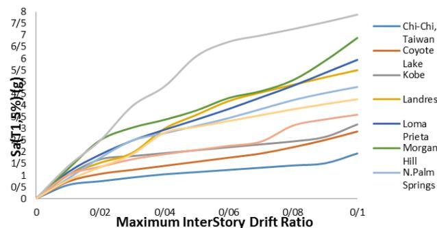
Figure 4. Category of IDA curves for four floor frame with 6 spans of 4 m and compressive strength of 21 MPa.
