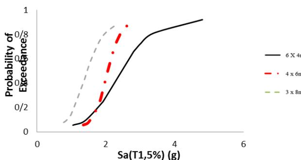
Figure 32. Fragility curves for frames with 4 floor structure with compressive strength of 21 MPa in CP performance level.
