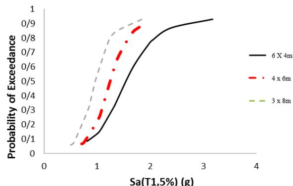
Figure 28. Fragility curves for frames with 4 floor structure with compressive strength of 18.58 MPa in LS performance level.
