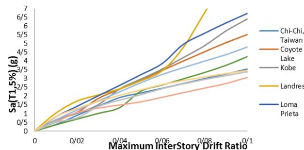
Figure 7. Category of IDA curves for four floor frame with 4 spans of 6 m and compressive strength of 21 MPa.
