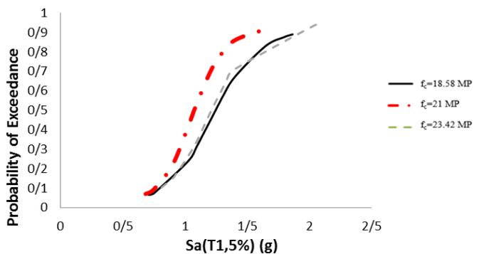
Figure 22. Fragility curves for four floor frame with 4 spans of 6 m in LS performance level.
