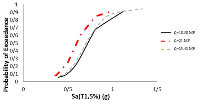
Figure 21. Fragility curves for four floor frame with 4 spans of 6 m in IO performance level.
