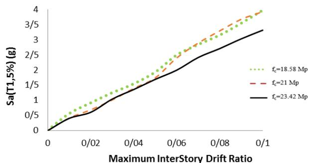
Figure 14. Mean values of IDA curves of four floor frame with various compressive strengths for 3 spans of 8 m.
