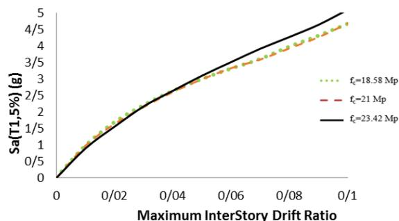
Figure 12. Mean values of IDA curves of four floor frame with various compressive strengths for 6 spans of 4 m.
