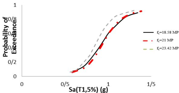
Figure 18. Fragility curves for four floor frame with 6 spans of 4 m in IO performance level.
