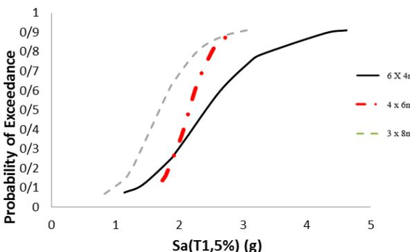
Figure 29. Fragility curves for frames with 4 floor structure with compressive strength of 18.58 MPa in CP performance level.
