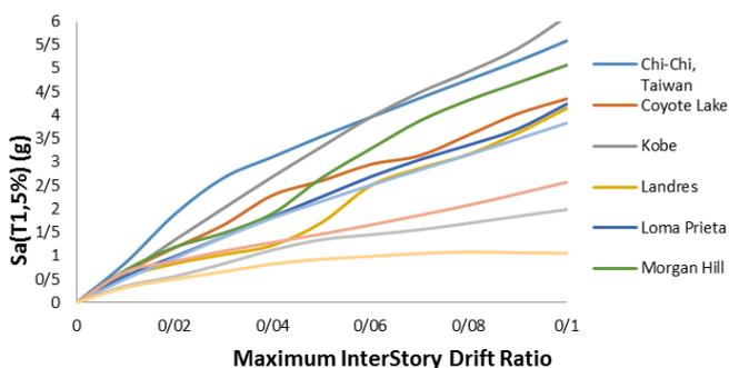
Figure 9. Category of IDA curves for four floor frame with 3 spans of 8 m and compressive strength of 18.58 MPa.
