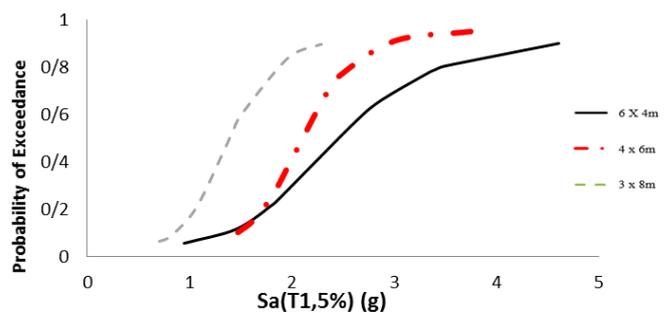
Figure 35. Fragility curves for frames with 4 floor structure with compressive strength of 23.42 MPa in CP performance level.
