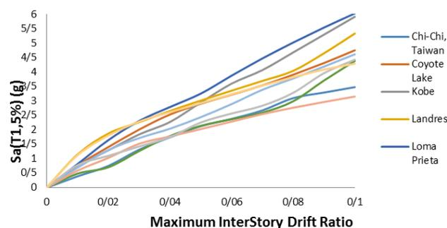
Figure 6. Category of IDA curves for four floor frame with 4 spans of 6 m and compressive strength of 18.58 MPa.
