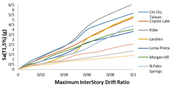
Figure 10. Category of IDA curves for four floor frame with 3 spans of 8 m and compressive strength of 21 MPa.
