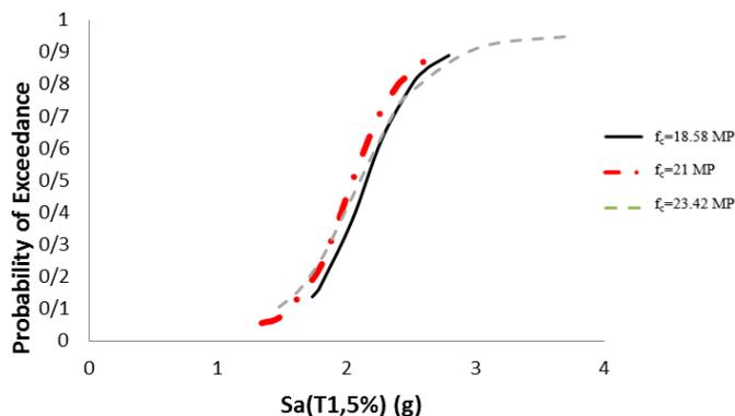
Figure 23. Fragility curves for four floor frame with 4 spans of 6 m in CP performance level.
