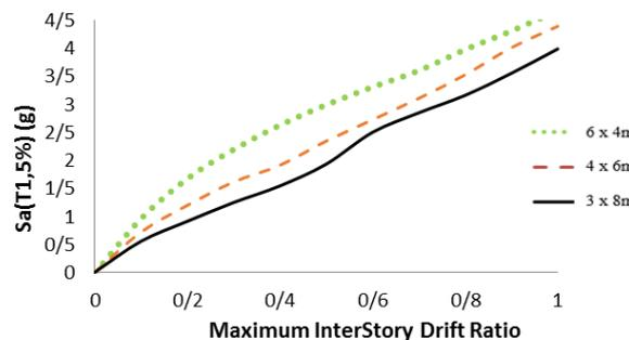
Figure 15. Mean values of IDA curves of four floor frame for spans with various dimension and comp. strength of 18.58 MPa.
