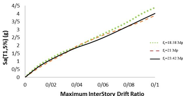
Figure 13. Mean values of IDA curves of four floor frame with various compressive strengths for 4 spans of 6 m.
