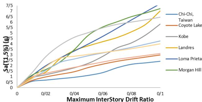
Figure 5. Category of IDA curves for four floor frame with 6 spans of 4 m and compressive strength of 23.42 MPa.
