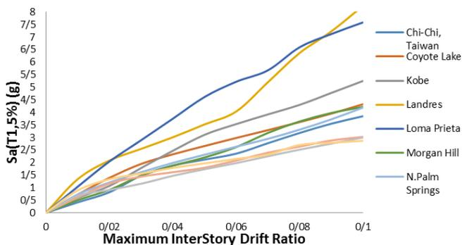
Figure 8. Category of IDA curves for four floor frame with 4 spans of 6 m and compressive strength of 23.42 MPa.
