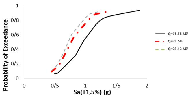
Figure 25. Fragility curves for four floor frame with 3 spans of 8 m in LS performance level.
