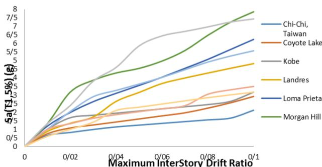
Figure 3. Category of IDA curves for four floor frame with 6 spans of 4 m and compressive strength of 18.58 MPa.
