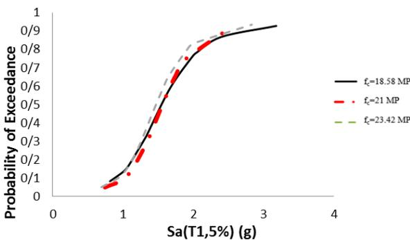
Figure 19. Fragility curves for four floor frame with 6 spans of 4 m in LS performance level.
