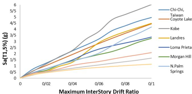
Figure 11. Category of IDA curves for four floor frame with 3 spans of 8 m and compressive strength of 23.42 MPa.
