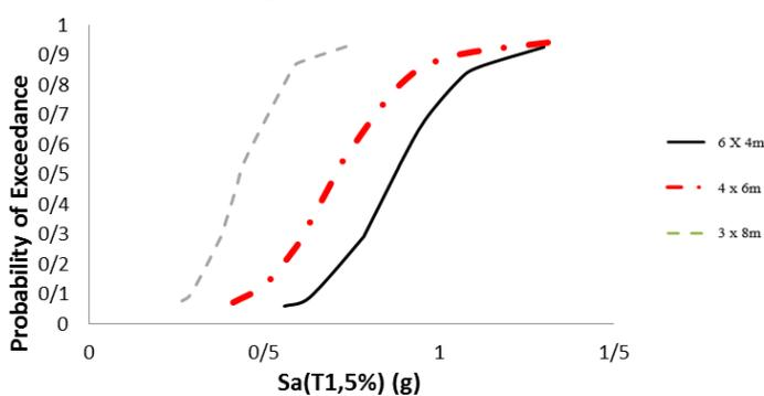
Figure 33. Fragility curves for frames with 4 floor structure with compressive strength of 23.42 MPa in IO performance level.
