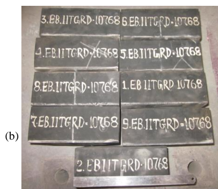
Figure 1. Details of prototype U-FREI: a) elastomer and fiber layers in the prototype U-FREI; b) specimens.
