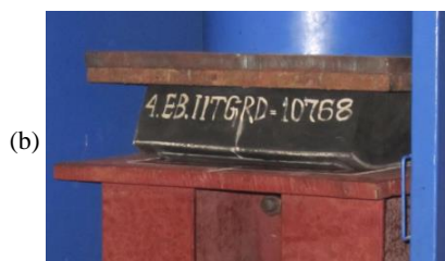
Figure 7. Deformed shapes of U-FREI at displacement amplitude of 80 mm and vertical force equal to 350 kN: a) FE analysis result; b) experimental result.
