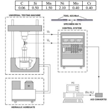
Figure 2. Overall scheme of the MTS testing system, /3/.
