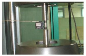
Figure 3. MTS extensometer.
