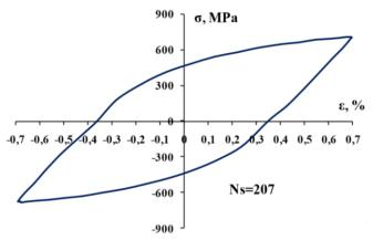
Figure 4. Example of stabilized hysteresis loop.
