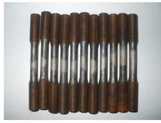
Figure 1. Round specimens prepared for LCF testing.
