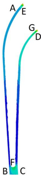
Figure 5. Stress path in the cement: AB-CD (external interface), and EFG (internal interface).
