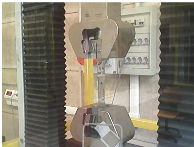
Figure 7. Specimen during the tensile shear test.
