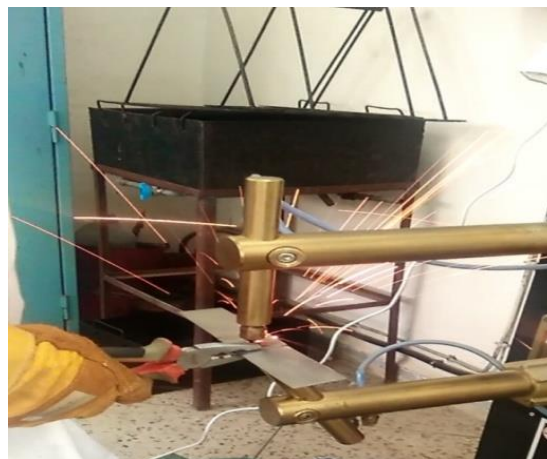
Figure 4. Specimens during resistance spot welding process.
