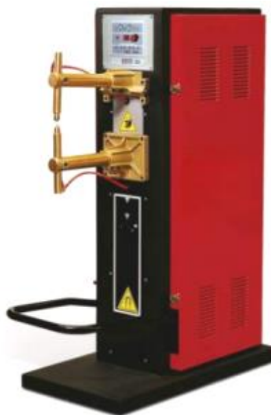
Figure 3. THI 50 Digit resistance spot welding machine.
