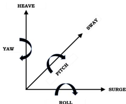
Figure 2. DOF in TLP motion (modified from /7/).
