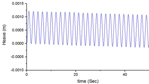
Figure 6. Decay test response obtained in heave DOF.
