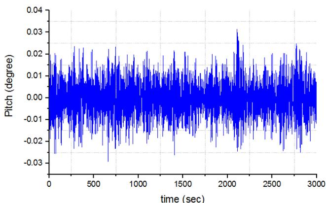
Figure 11. Response for pitch motion of TLP ( $H_s = 5$  m,  $T_z = 7$  s).
