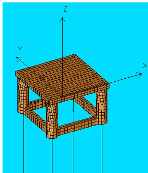
Figure 5. Meshed numerical model of ISSC TLP with 4 sets of tethers.
