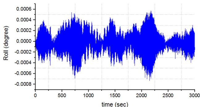
Figure 10. Response for roll motion of TLP ( $H_s = 5$  m,  $T_z = 7$  s).
