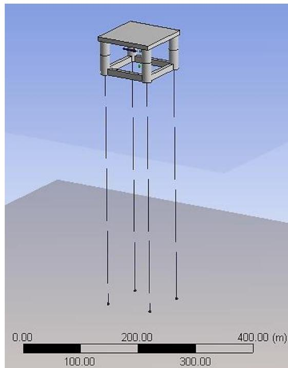
Figure 4. ISSC TLP modelled in ANSYS® AQWA module.
