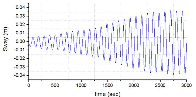
Figure 8. Response for sway motion of TLP ( $H_s = 5$  m,  $T_z = 7$  s).
