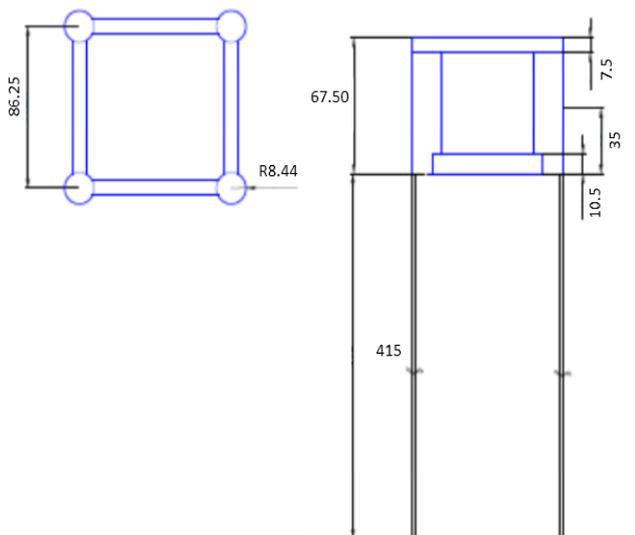
Figure 3. Configuration of the TLP model (modified from /12/, dimensions are in m).
