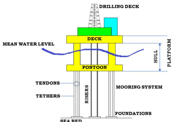
Figure 1. Schematic diagram of a TLP (modified from /6/).
