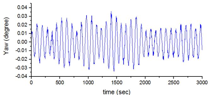
Figure 12. Response for yaw motion of TLP ( $H_s = 5$  m,  $T_z = 7$  s).
