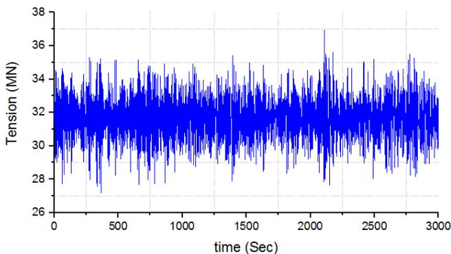
Figure 13. Variation of tether tension in legs of TLP ( $H_s = 5$  m,  $T_z = 7$  s).
