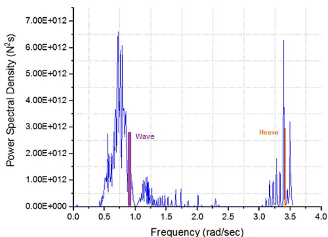
Figure 16. PSD for tether tension observed in the legs of the TLP.
