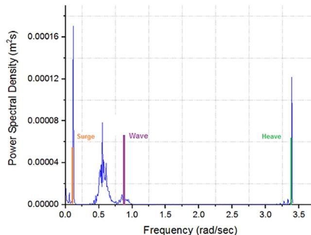
Figure 15. PSD for heave DOF of the TLP.
