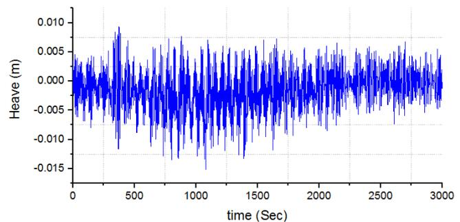
Figure 9. Response for heave motion of TLP ( $H_s = 5$  m,  $T_z = 7$  s).
