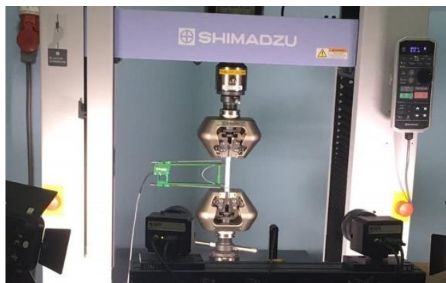
Figure 1. Setup of the cameras and extensometer.
