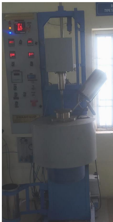
Figure 3. Stir casting setup (courtesy of Sai Ram College of Engineering, Chennai).
