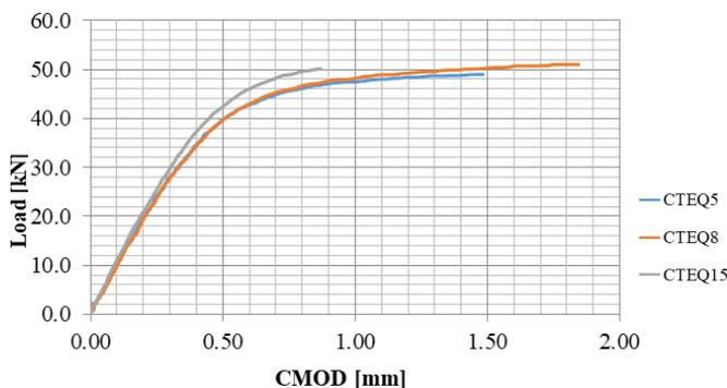
Figure 5. CMOD comparison for C(T)50 specimens at -60 °C and 0.5 mm/min displacement rate.
