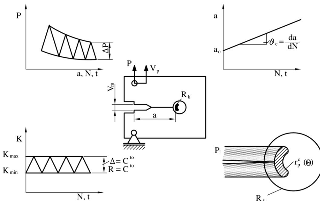
Figure 2. Illustration of fatigue crack growth at constant range ( $\Delta K = \text{const.}$ ) under limited yield condition, /26/.
