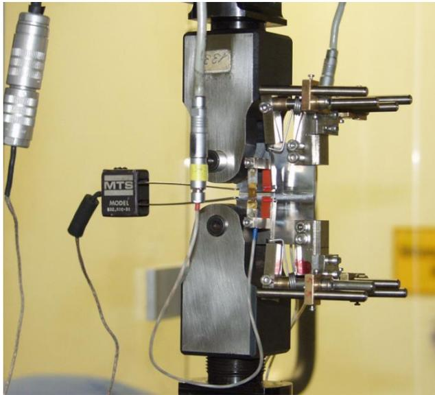
Figure 3. Experimental setup for C(T)50 specimen tests.
