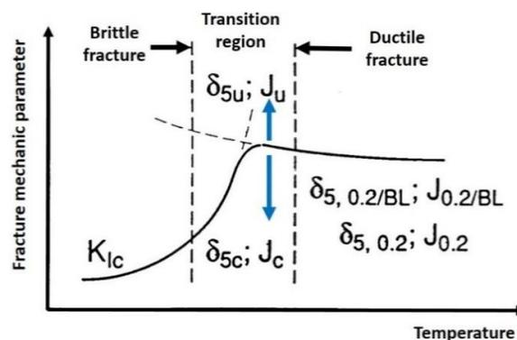
Figure 1. Influence of temperature on the selection of relevant fracture mechanics parameter, /22/.
