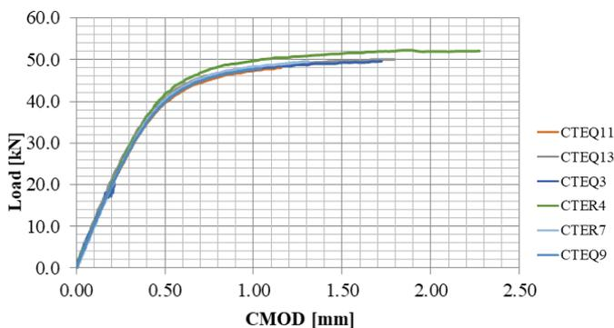
Figure 4. CMOD comparison for C(T)50 specimens at -60 °C and 0.02 mm/min displacement rate.
