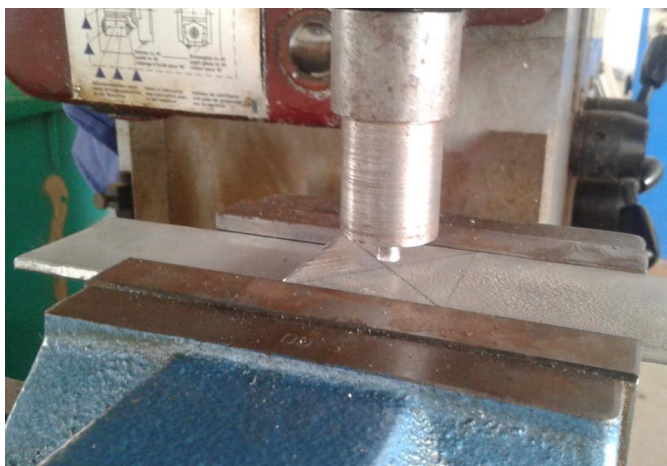
Figure 4. Specimens during the stir spot welding process.
