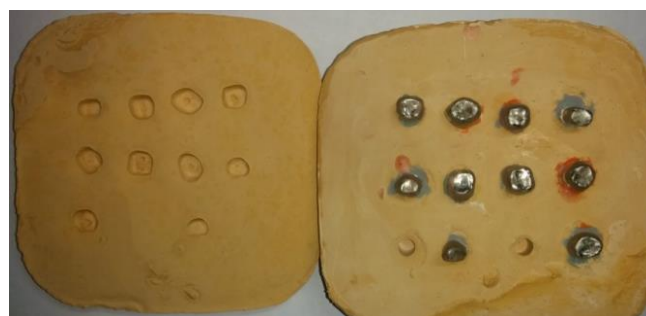
Figure 3. Forms from plaster: with imprints of teeth crowns (left), with fixed teeth (right).
