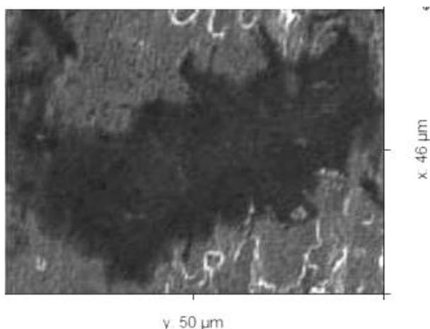
Figure 2b. SEM of Al6061-9 % graphite showing average particle size of graphite in an Al6061 matrix.
