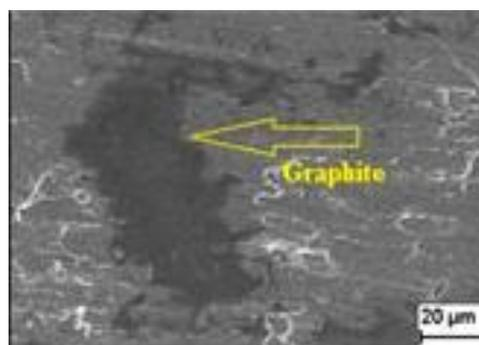
Figure 2a. SEM of Al6061-9 % graphite, demonstrating interface between matrix and reinforcement.
