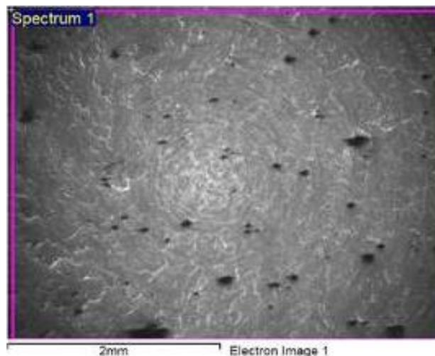
Figure 1a. SEM graph showing a distribution of graphite particles in Al6061-9 % graphite.
