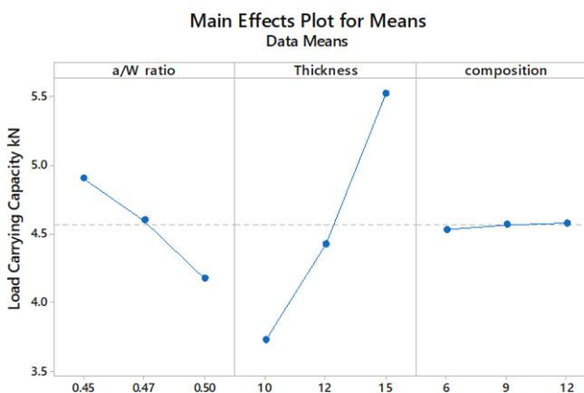
Figure 3a. Taguchi’s design results for load carrying capacity.
