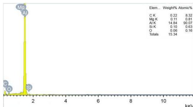
Figure 1b. EDX profile analysis of Al6061-9 % graphite surface.
