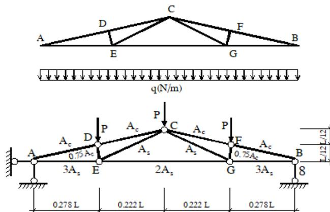
Figure 3. Schematic diagram of roof truss, /21/.
