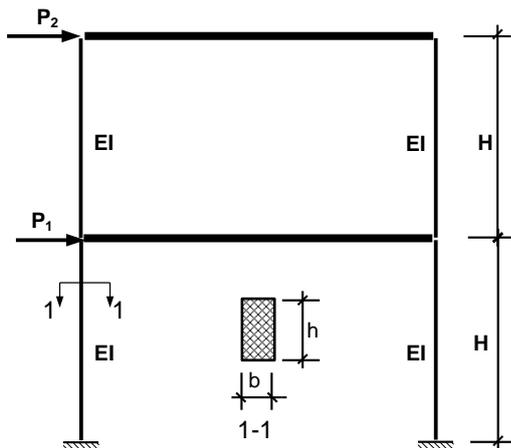
Figure 4. Two-story frame structural system.
