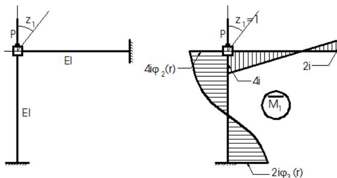
Figure 6. The primary structural frame system and bending moment diagram.
