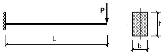
Figure 2. Cantilever beam subjected to tip load  $P$ .
