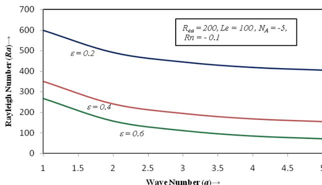
Figure 6. Variations of thermal Rayleigh number  $Ra$  with wave number  $a$  for medium porosity  $\epsilon = 0.2, 0.4 \text{ and } 0.6$ .
