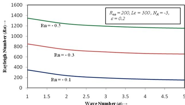
Figure 5. Variations of thermal Rayleigh number  $Ra$  with wave number  $a$  for nanoparticle Rayleigh number  $Rn = -0.1, -0.3, -0.5$ .
