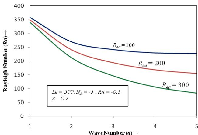
Figure 2. Variations of thermal Rayleigh number Ra with wave number a for values of AC electric Rayleigh number  $R_{ea} = 100, 200$  and  $300$ .
