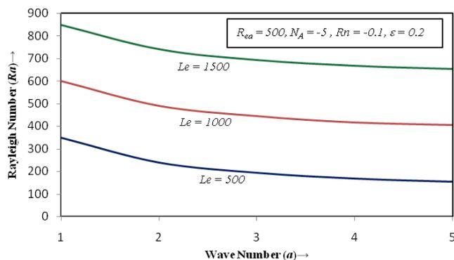
Figure 3. Variations of thermal Rayleigh number Ra with wave number  $a$  for Lewis number  $Le = 500, 1000, \text{ and } 1500$ .
