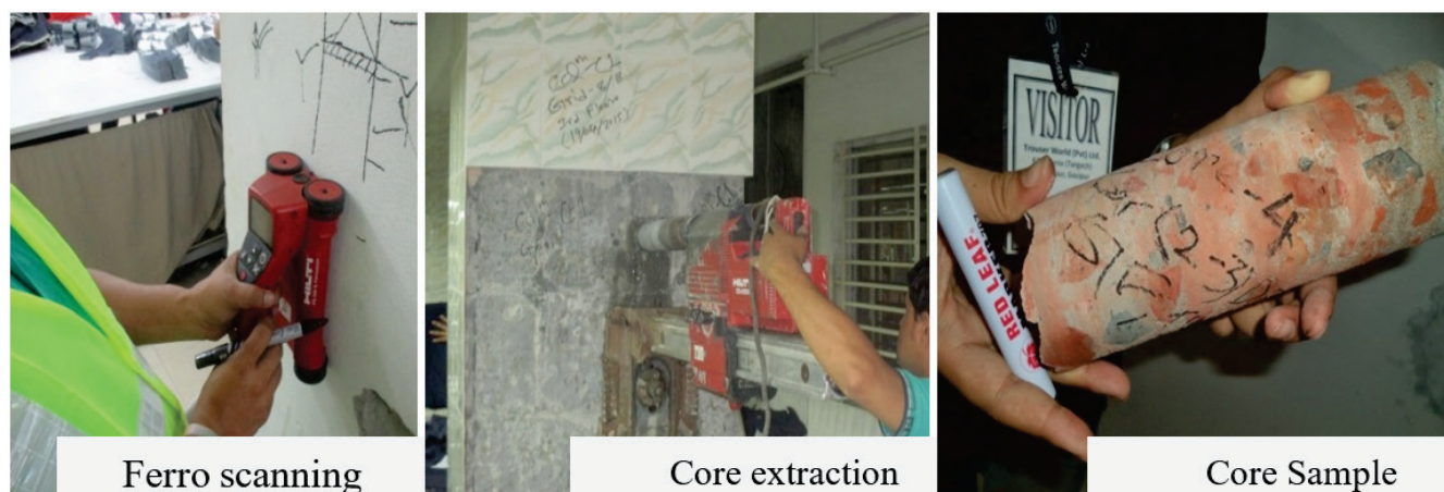
Figure 1. Concrete core extraction test.
