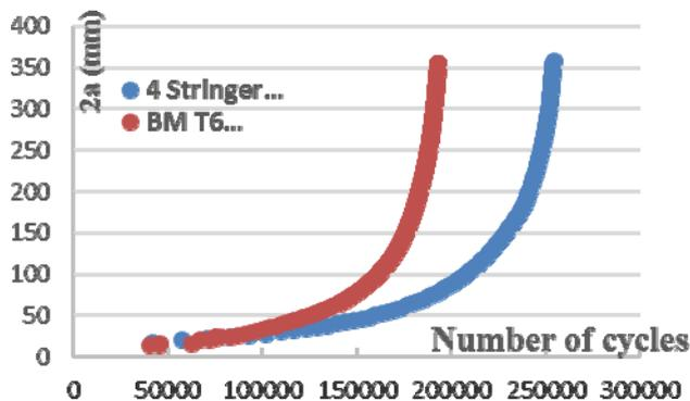
Figure 6. Number of cycles for base metal plate obtained in the experiment and 4-stringer plate obtained in simulation by XFEM.
