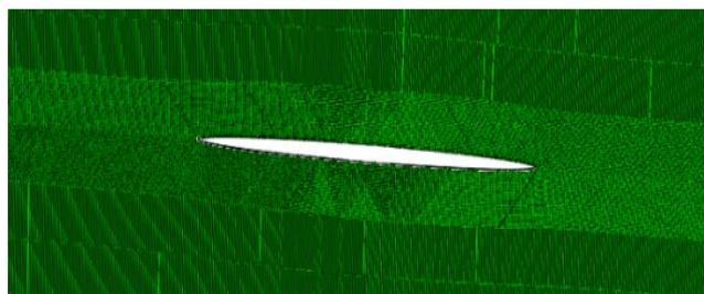
Figure 3. Crack in base metal plate after 260 steps of propagation ( $2a = 275$  mm).
