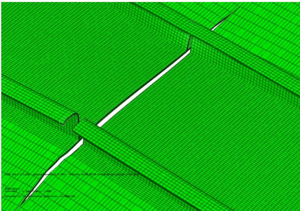
Figure 5. Crack after 160 steps of propagation.
