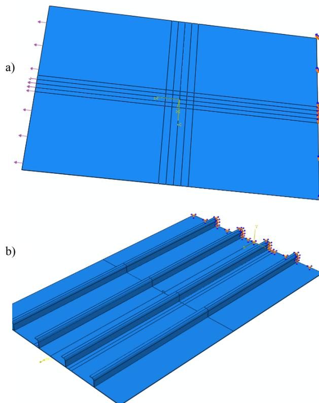
Figure 2. FE model of base metal plate with initial crack, a) simple panel, base metal, b) integral 4-stringer panel.
