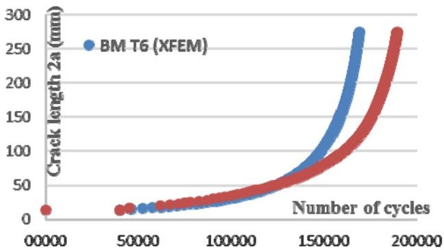
Figure 4. Numbers of cycles obtained in experiment and XFEM simulation (base metal T6).
