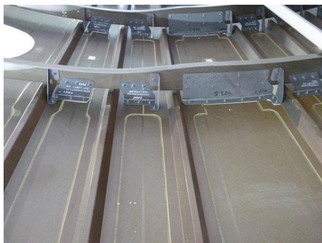
Figure 1. Integral skin-stringer structure of the fuselage.
