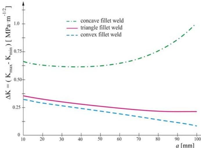
Figure 4. Variation of  $\Delta K = K_{max} - K_{min}$  with crack length for  $F_{min} = 1$  kN to  $F_{max} = 10$  kN.
