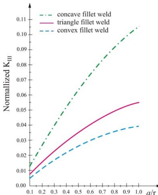
Figure 3. Normalized Mode III SIF vs. normalized crack length.
