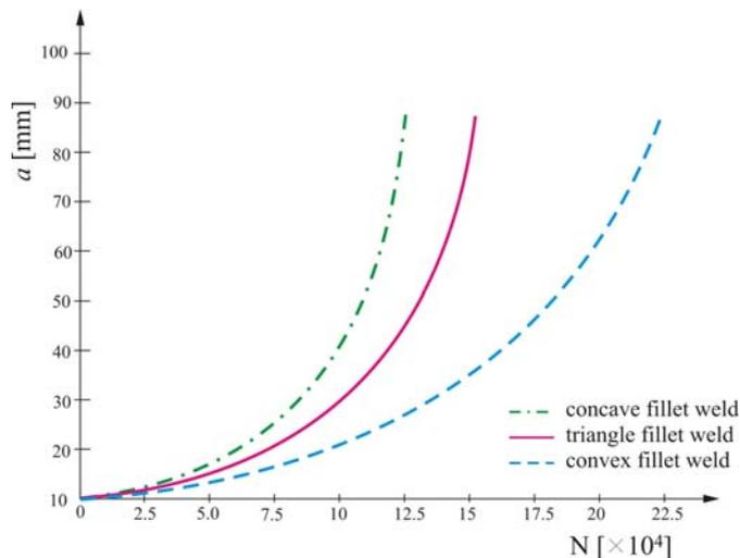
Figure 5. Fatigue crack growth curve: crack length vs. number of load cycles,  $a$  vs  $N$ .
