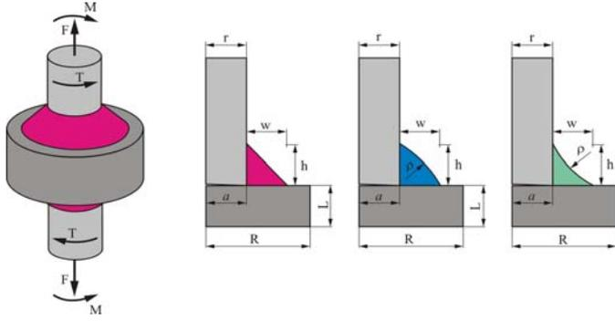
Figure 1. Fillet welds in cylindrical parts; loading and geometry.
