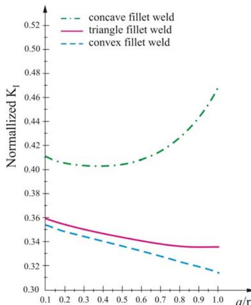
Figure 2. The normalized Mode I SIF vs. normalized crack length.
