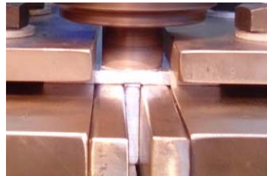
Figure 3. Penetration of the tool mandrel into the work plate.
