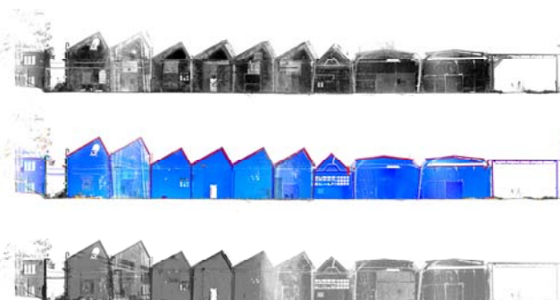
Figure 4. Orthophotos of northeast facade of Forge Workshop – model with infrared texture, range map, and side light.
