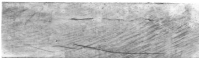
Figure 1. Cracks in welded joint between shell and tank head.
