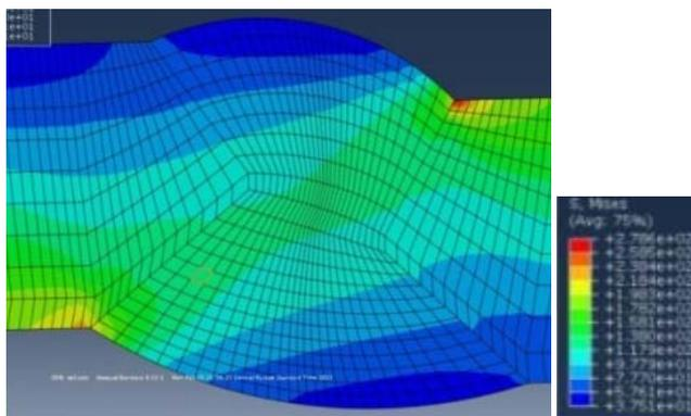
Figure 3. Stress distribution in the cross section of the welded joint with defects.
