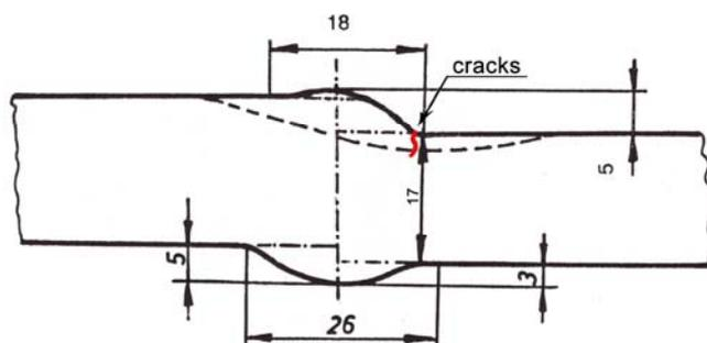
Figure 2. Cross section through the weld with cracks.
