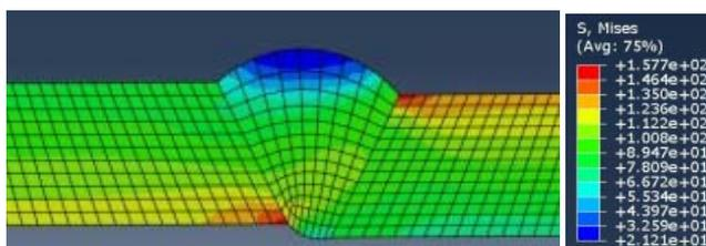
Figure 4. Stress distribution in the cross section of the welded joint with acceptable linear misalignment.
