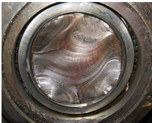
Figure 12. Failure section towards the bearing. Slika 12. Presek loma prema ležištu
