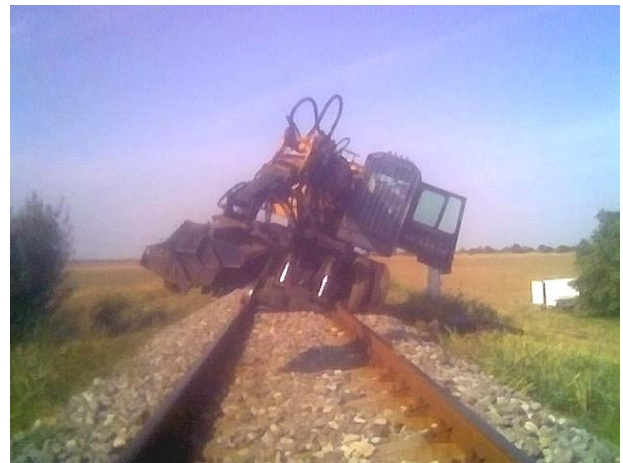
Figure 4. Overall position after the breaking of front left rail axle. Slika 4. Položaj nakon loma prednje leve vagonсke osovine
