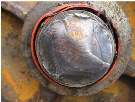
Figure 11. Section of fracture towards the rail wheel. Slika 11. Presek loma prema vagonском тоčku
