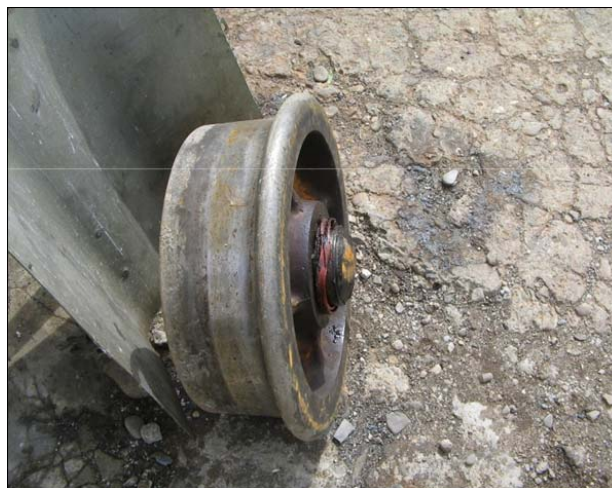
Figure 10. Fracture of the rail axle, near to the rail wheel. Slika 10. Lom vagonke osovine, blizu vagonkog točka
