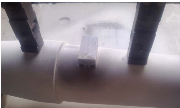
Figure 16. Magnetic particle inspection of T3500 railway axles. Slika 16. Ispitivanje T3500 vagonskih osovine magnetnim česticama
