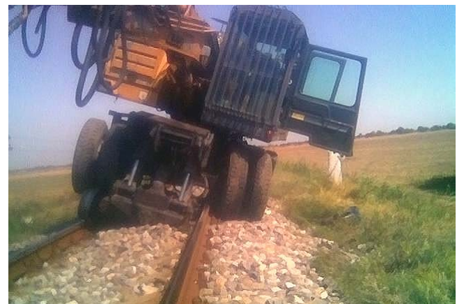
Figure 5. Position after the left rail axle failure – front view. Slika 5. Položaj nakon loma leve vagonсke osovine – s preda
