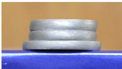
Figure 17. Pieces with 1.5 h_0/d_0 ratio of the three different passes, from top: eight, four and one pass (largest diameter).
