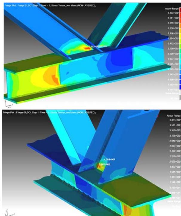
Figure 7. Imperfections type 1, FEM results, Von Mises stresses.
