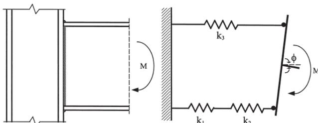
Figure 1. Welded beam to column joint – mechanical model, /3/.
