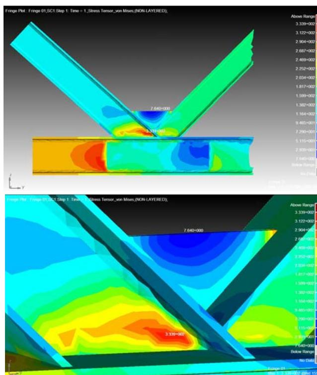
Figure 10. Strengthened joint, FEM results, Von Mises stress.
