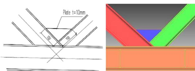
Figure 9. Strengthened joint – geometry.
