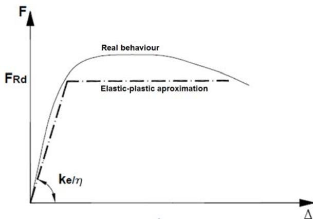
Figure 2. Idealizations of the force-deformation curve /2/.
