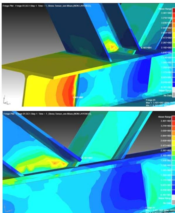
Figure 8. Imperfections type 2, FEM results, Von Mises stress.
