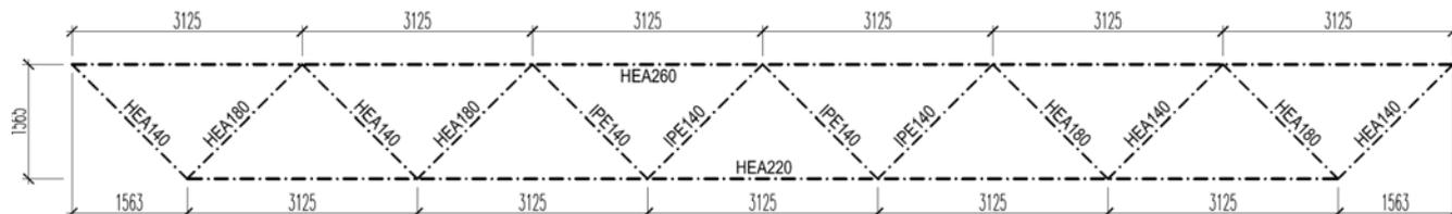
Figure 4. Geometry of the truss beam.
