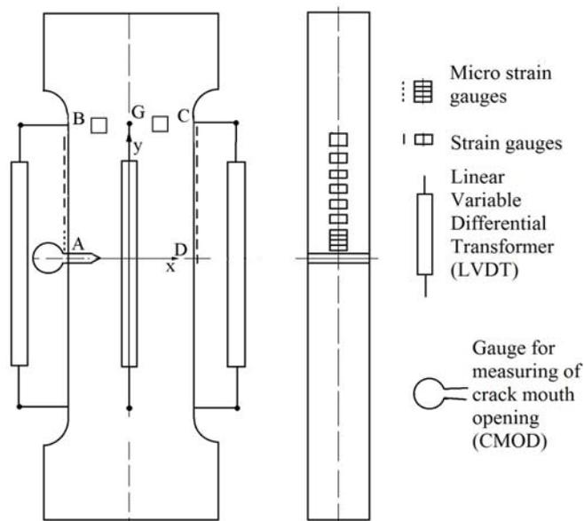
Figure 3. Instrumentation for tension tests of the edge cracked specimen.
