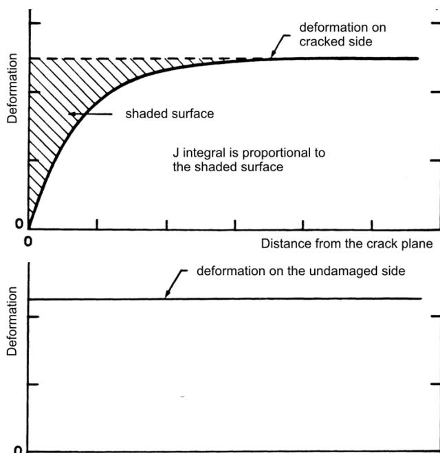
Figure 8. Deformations on the crack side and on the smooth side: interpretation of the J integral, /1/.
