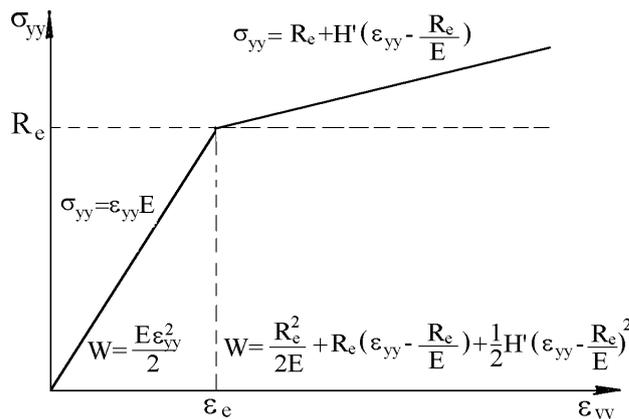
Figure 4. Stress-strain curve for a hardening material.
