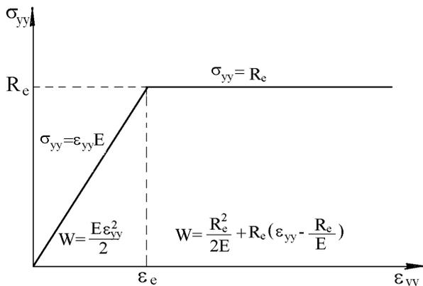
Figure 2. Stress-strain curve for elastic-ideally plastic material behaviour.
