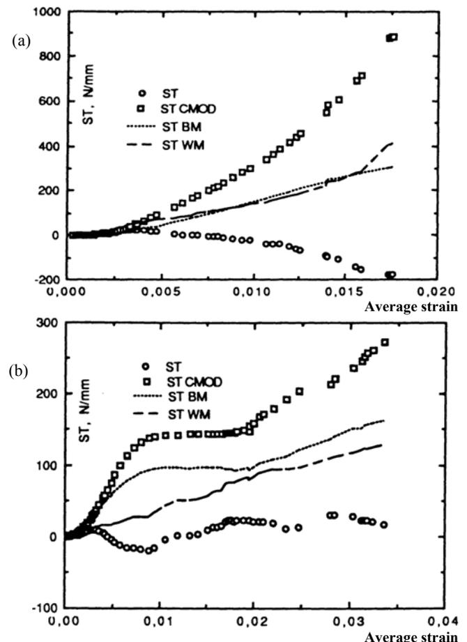
Figure 5. ST component of J integral, a) under-, b) over-matching, /9/ Slika 5. ST komponenta J integrala, a) ander-, b) over-mećing, /9/
