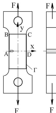
Figure 1. Contour  $\Gamma$  on a tensile specimen with an edge crack.
