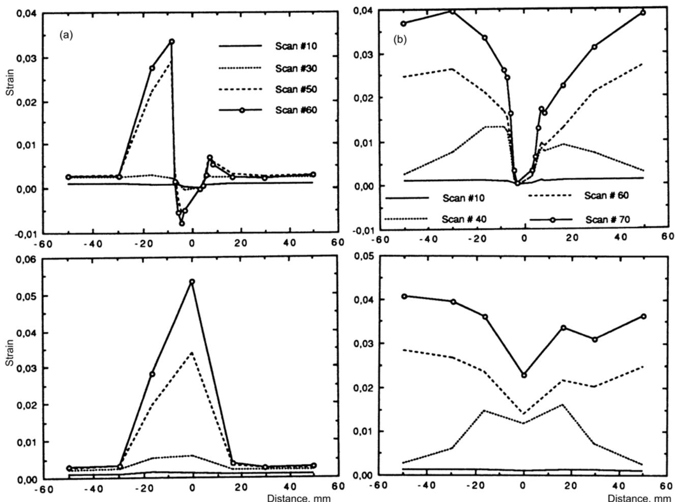
Figure 7. Deformation on the crack side and on the smooth side: a) under-matching, b) over-matching, /9/
