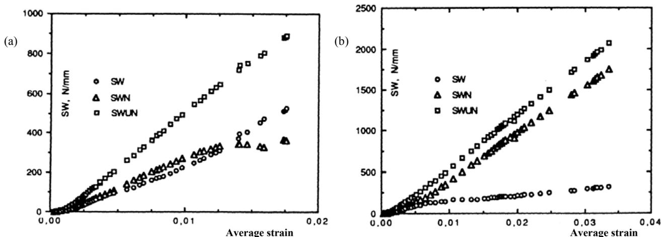
Figure 6. SW component of J integral: a) under-, b) over-matching, /9/
