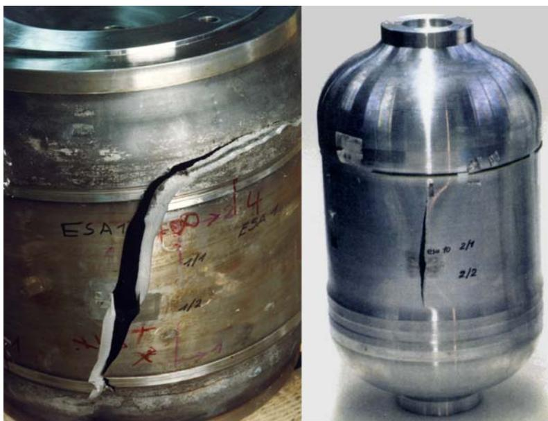
Figure 9. Fractured cylinder specimens with surface crack.
