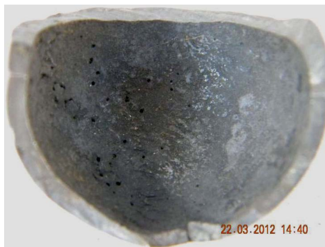
Figure 4. Defect of the ball by breaking of the outer layer.
