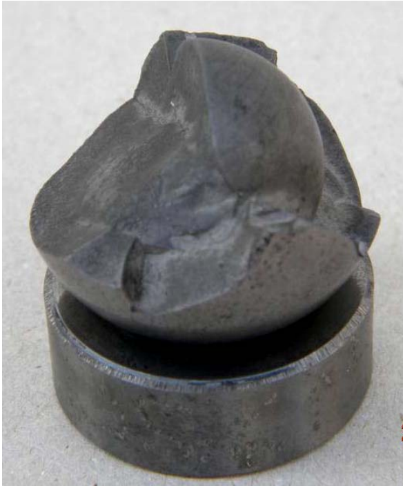
Figure 5. Defect of the ball made by the breaking of the outer layer and a piece of initial ball.
