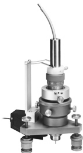
Figure 6. Measuring device for HDM (RS 200 Milling Guide by Micro Measurements). Slika 6. Uredaj za merenje za HDM (RS 200 Micro Measurements)
