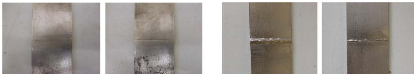
Figure 2. Right side and the reverse side of a smoothed specimen and of a classic welded specimen. Slika 2. Desna strana i suprotna strana glatkog uzorka i klasičnog zavarenog uzorka
