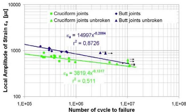
Figure 10.  $\epsilon_a-N$  fatigue curves between cruciform and butt joints.
