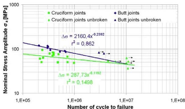
Figure 9.  $\sigma_a-N$  fatigue curves of cruciform and butt joints.
