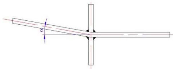
Figure 3. Distortion angle on the specimen after the weld process.
