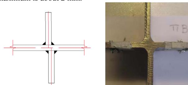
Figure 4. Some welded joints present flange misalignment.
