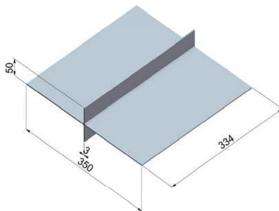
Figure 1. Ti6Al4V welded plate, dimensions of plates and flanges.
