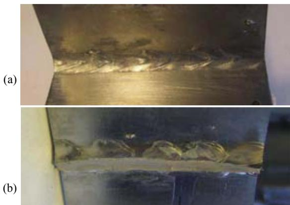
Figure 8. Weld cords: a) A and B plates; b) C and D plates.
