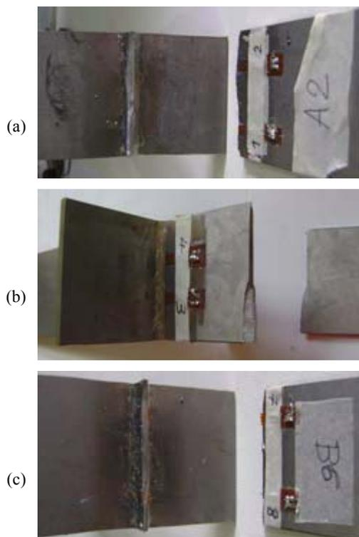
Figure 5. Three different fatigue fracture locations for the cruciform no-load carrying Ti6Al4V hybrid welded joints: (a) at the weld toe; (b) within the nominal zone; (c) within the HAZ.
