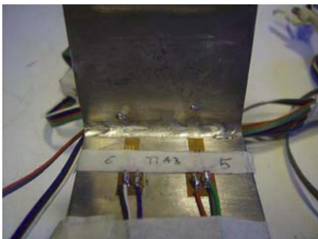
Figure 2. Disposition of strain gauges on the welded specimen.
