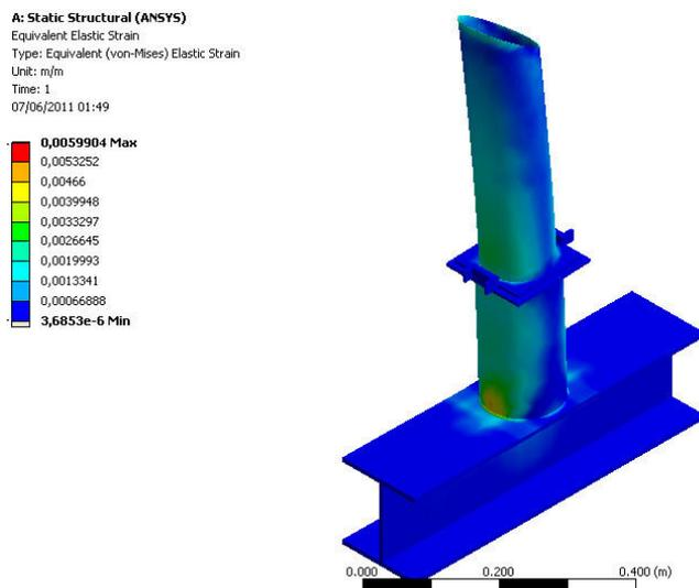
Figure 10. Equivalent (Von-Mises) stress distribution.
