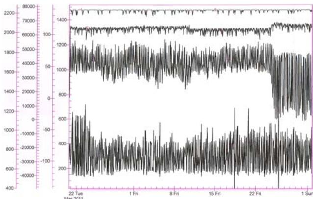
Figure 3. Pump speed, discharge pressure, overboard return flow and condensate pump flow.
