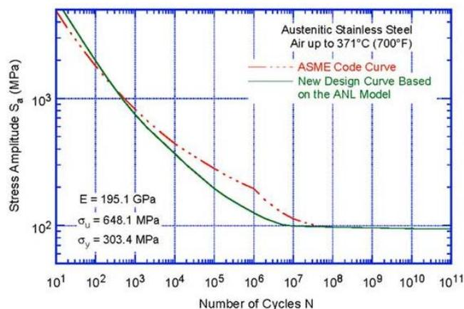
Figure 12. S-N curve for austenitic stainless steel not exceeding 371°C.
