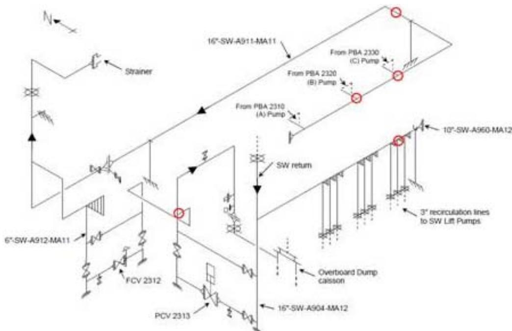
Figure 2. Schematic layout of seawater pipework in sub-cellar deck
