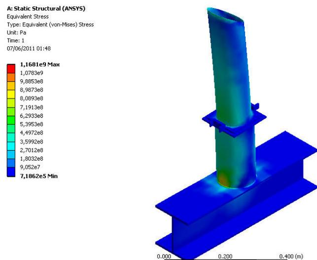
Figure 9. Equivalent (Von-Mises) stress distribution.
