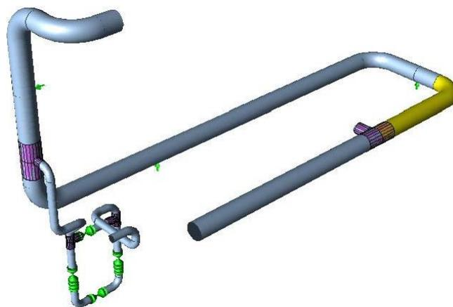
Figure 5. Layout of seawater cooling pipework.
