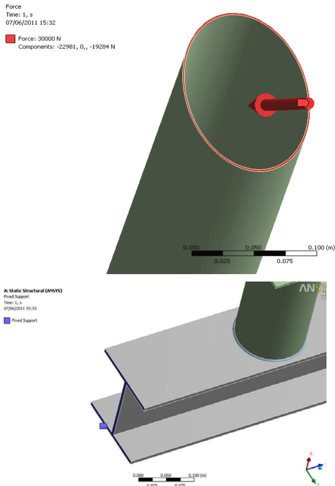
Figure 8. Boundary conditions (elbow force  $K = 31$  kN and support fixed end).
