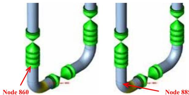
Figure 7. Maximum load force in node 860 and stress in node 885.
