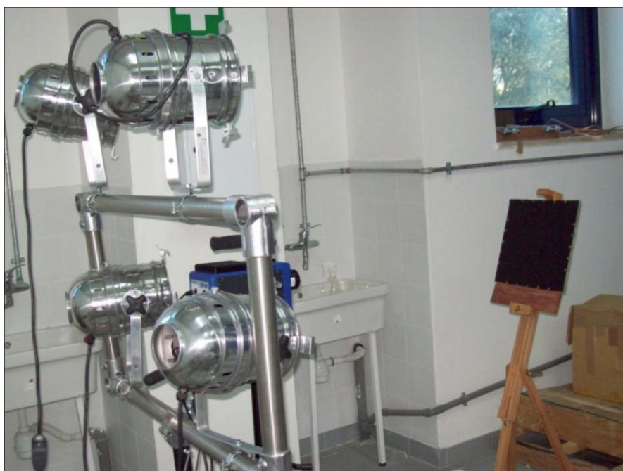
Figure 1. Thermographic set-up for specimens 1 and 2.
