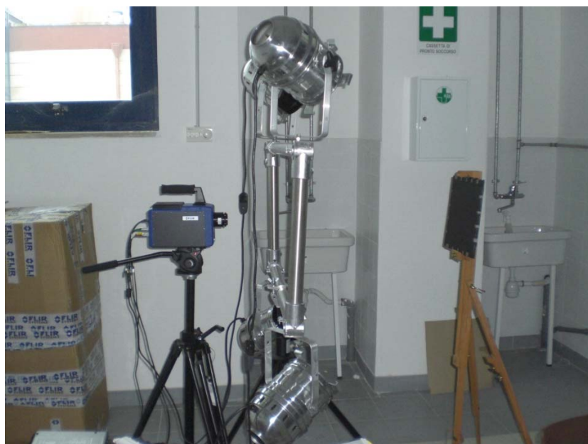
Figure 3. Thermographic set-up for specimen 3.
